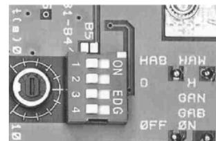
Use the potentiometer to the left of the switches to set the GAN and GAB times steplessly from 0.1 s ... 10 s.
